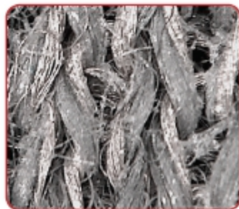
Microscopic view of Carraro Conductive Suit with helically wound silver yarn (shiny silver) in comfortable knit fabric.
