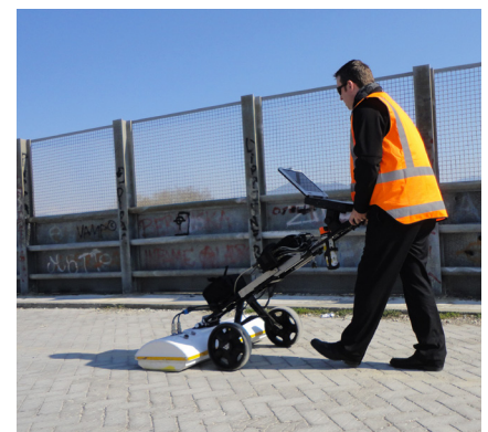
RIS Hi-BrigHT: pavement surveying
