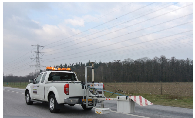
RIS Hi-Pave with high and medium frequency antennas
