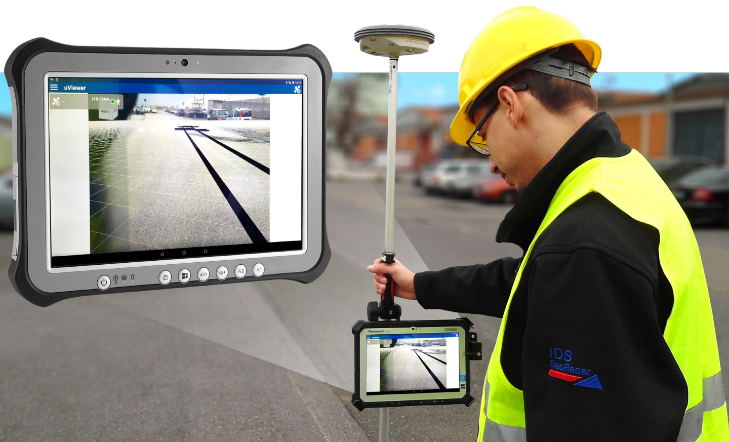
Visualisation of underground detected objects in Augmented Reality
